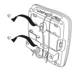
7. On the base, pull the handset retainer out of the slot. Rotate clockwise 180°.
